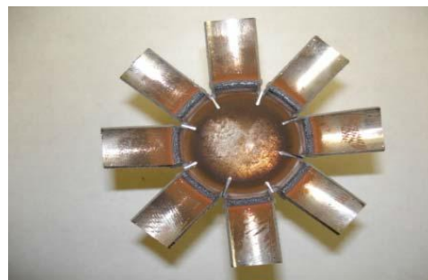
Figure 6 – Tulip test on tube to tenon weld
