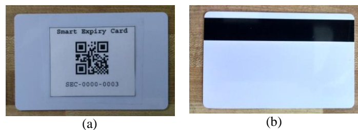
Figure 5. Smart-expiry magnetic card: (a) Top view - containing the card ID in QR code and in English letters; (b) Bottom view - containing the card ID written in the magnetic strip.
