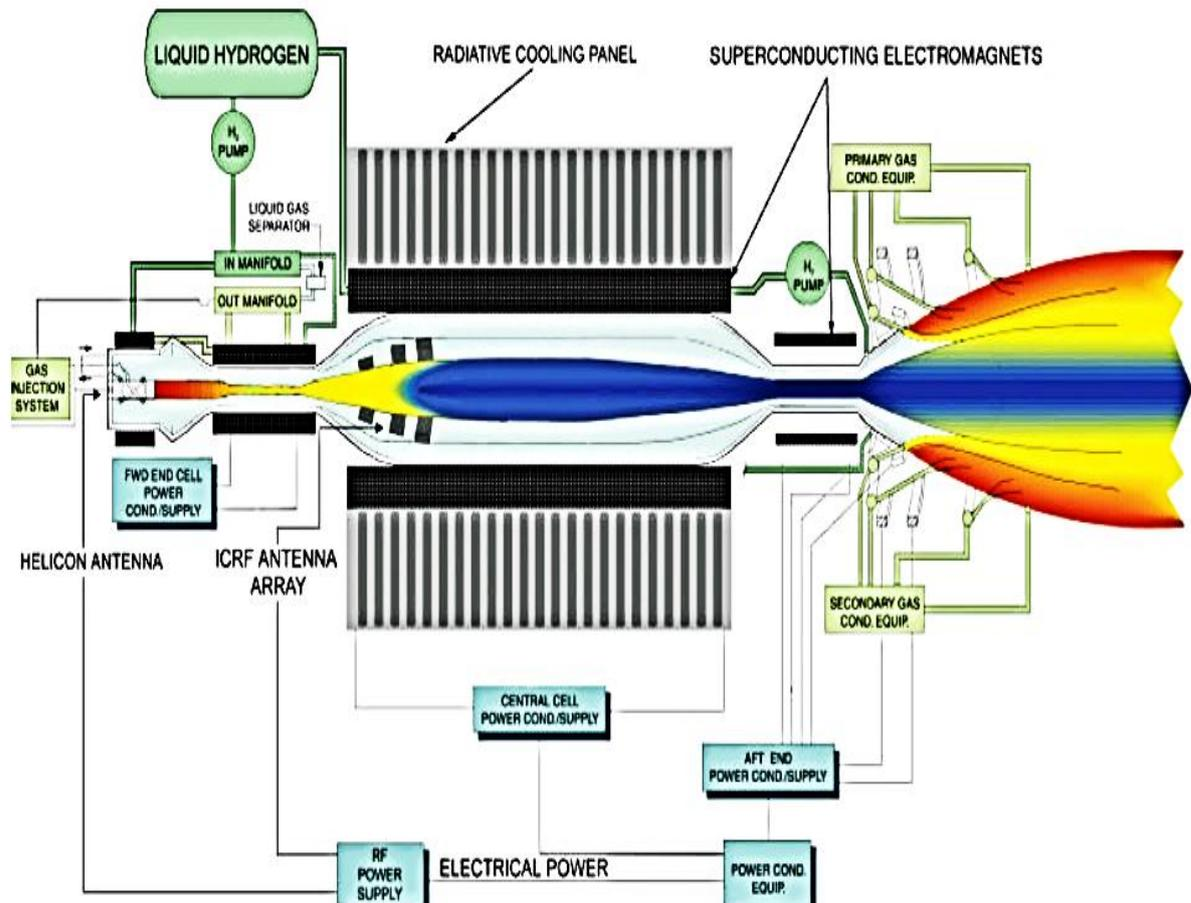
(Fig 1: The VASIMR concept; Source: AIAA 2000-3756 *The Physics and Engineering of the VASIMR Engine*)
