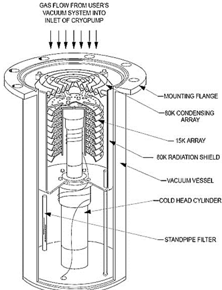
(Fig 4: Cutaway view of a typical Cryo-Torr cryogenic pump; Source: Cryo-Torr High Vacuum Pump Installation, Operation and Maintenance Instructions, 8040613, Rev. (4/2001))
