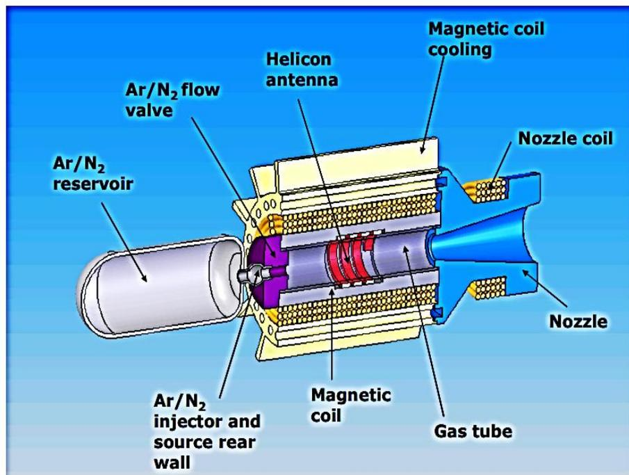
(Fig3: Scheme of HPH.COM helicon thruster; Source: D.J. Santeler et al., *Vacuum Technology and Space Simulation*, NASA SP-105)
