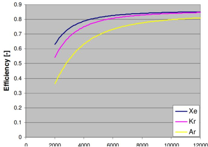
(Fig 2: Representative ion thruster efficiency,  $\eta$ , for Xenon (Xe), Krypton (Kr), and Argon (Ar).; Source; *Xe Ion Propulsion for Orbit Transfer* by V. K. Rawlins, M. J. Patterson, and R. P. Gruber)
