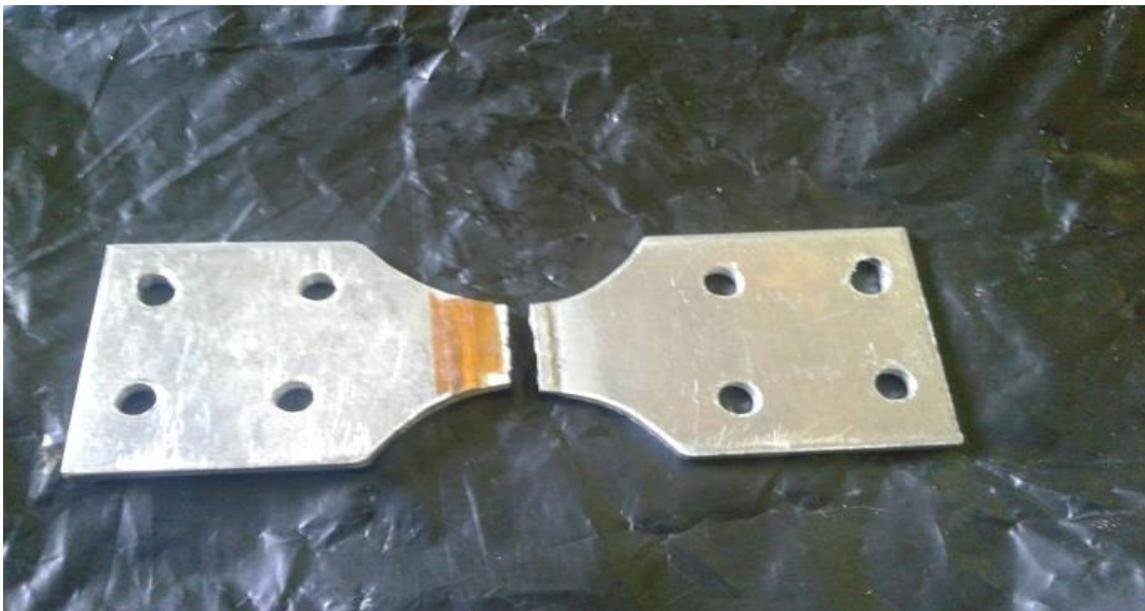
**Figure 13:** Specimen after Fatigue Failure
