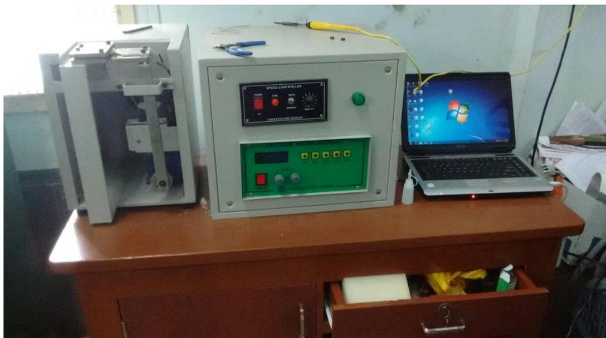
**Figure 5:** Low cycle Fatigue Measurement Instrument
