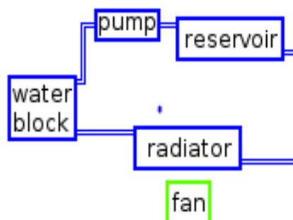
Figure 3: Schematic of a regular liquid cooling setup for PC's.
