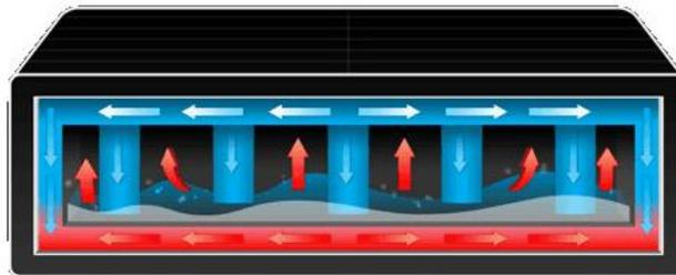
Figure 2: <https://www.maketecheasier.com/what-is-vapor-chamber-cooling/>. This image depicts the heat flow inside the vapor chamber when heat waves are passed through it.
