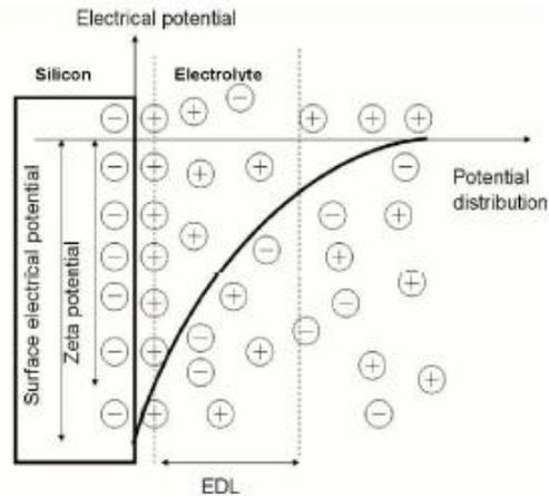
Figure 6: Electric double layer (EDL) by the wall
