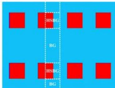
Figure 5: This image shows the heatmap of a conventional multicore microprocessor. The red area are hotspots which are the cores of the microprocessor.
