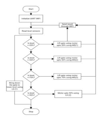
Fig 2: The Flow charts describes the different levels reached by the water and the level to which the gate is to be opened.
