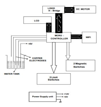
Fig 1 : The above figure shows the block diagram of dam gate resource analysis
