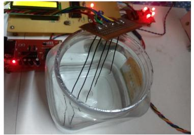
Fig 4:Copper electrodes as sensing elements
