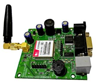
Figure 1.1c: GSM module
