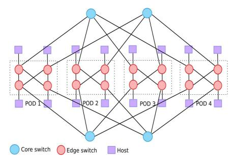
Fig. 6. An example of F2Tree DCN with K = 6. It consists of 26 switches, 24 hosts, and 90 links.
