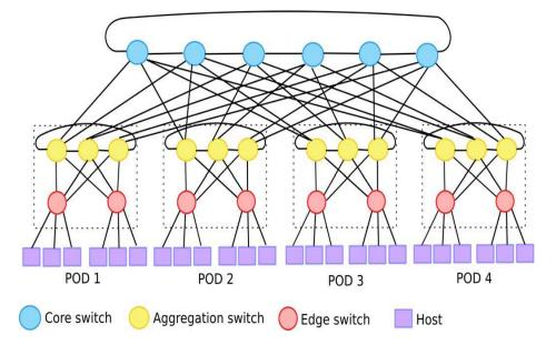
Fig. 5. An example of a Fat-Tree DCN with K = 4. It consists of 20 switches, 16 hosts, and 48 links.
