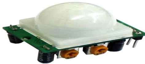
Fig 5.1 : Structure of PIR sensor
