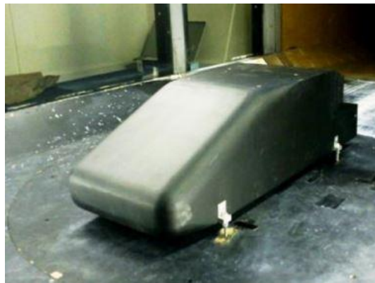
Figure 5 tapered windsor body for wind tunnel body
