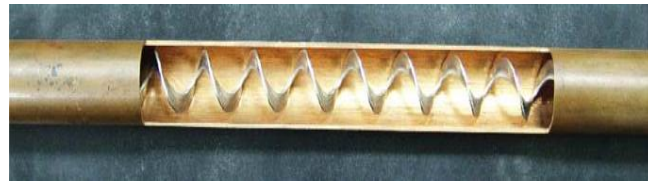
Fig. 2 Helical twisted tape without core rod
