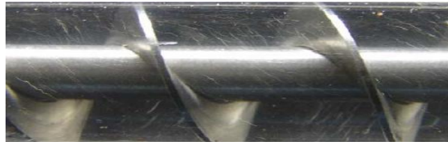
Fig. 1 Helical twisted tape with core rod
