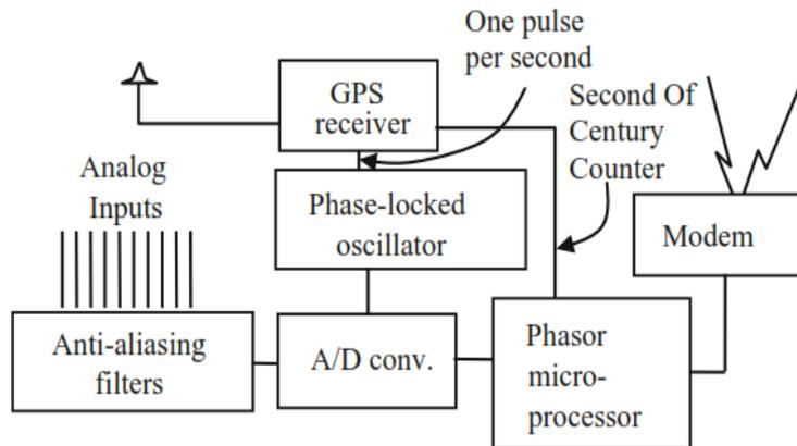
Figure 2. Block Elements of PMU[5]
