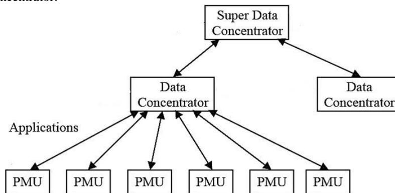
Figure 1. Three Layered structure of WAMS[3]
