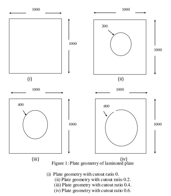
Four types of boundary condition namely FFFC, FCFC, CCCC and SSSS (where F, C and S stand, respectively, for a free, a clamped, a simply supported edge) are considered in order to examine the effect of boundary condition on the fundamental natural frequency of a square graphite epoxy laminate with a centrally located circular cutout.
