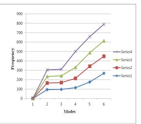
Figure 2.2: Graph between Frequency and Modes under FCFC boundary Conditions
