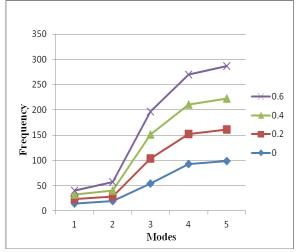
Figure 2.1: Graph between Frequency and Modes under FFFC boundary Conditions
