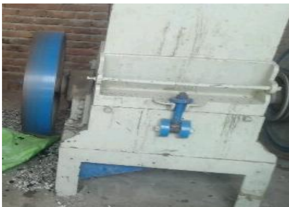
Figure 1 Shredding of Plastic of Waste
