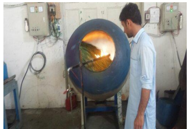
Figure 2 Moisture Removal Process from Plastic Waste
