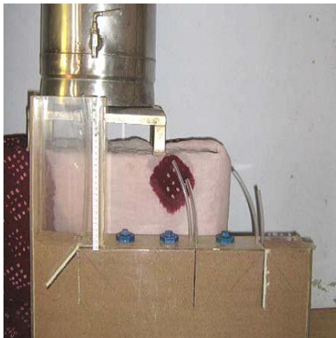
Figure-12. Variation of Uplift Pressure when upstream pile is inclined towards upstream
