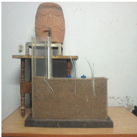
Figure-13. Variation of Uplift Pressure when upstream pile is inclined towards downstream
