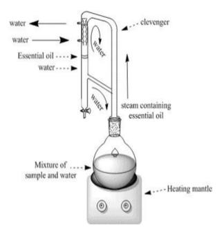
**Procedure:**25 gm crushed sample (Eucalyptus, Karanja, Basil) leaves taken into round bottom flask and 500ml water into it. Distill it till we get the constant volume of volatile oil in the distillation trap. Once optimum oil is collected in the trap, measure the volume of oil recovered in trap. Calculate percentage of oil on the basis of volume of the sample.
