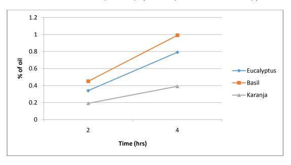
Essential Oil obtained is negligible before the components of the oil reach to their boiling point. After reaching to their boiling points Essential Oil is obtained. From the graph we can see that Basil oil is more as compared to Eucalyptus and Karanjaoil. Whereas karanja leaves contains lesser amount of essential oil.
