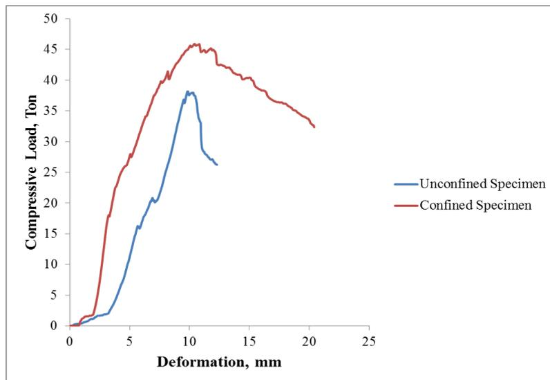
Figure 5: Load vs. Deformation Curve of Unconfined and Confined Specimen
