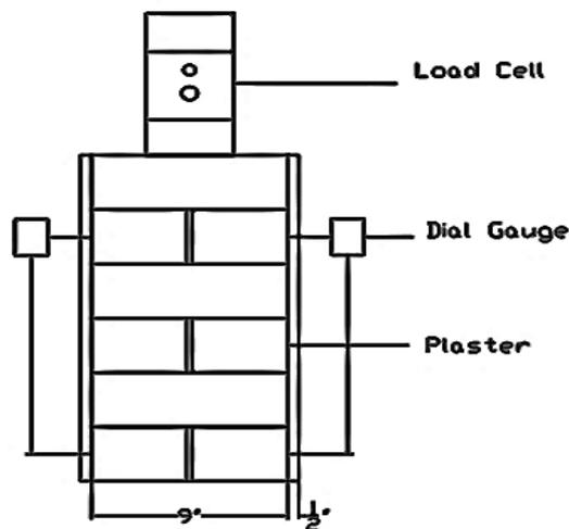
**Figure 3: Experimental Setup for testing the specimen under compression**
