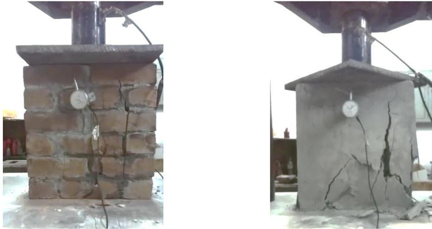
Figure 4: Testing of brick masonry prism (a) Unconfined; without wire mesh (b) Confined; with wire mesh
