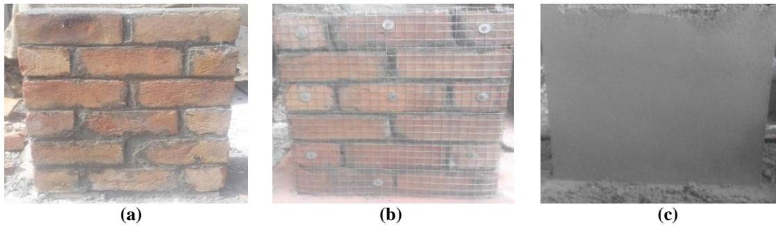
**Figure 2: Samples (a) Unconfined Prism (UP) (b) Steel wire mesh applied to prism (c) Plastered prism**
