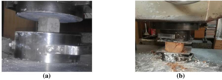
**Figure 1: Compressive strength test (a) Mortar (b) Brick**
