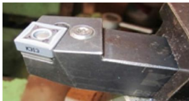
Figure 3. Uncoated carbide with designated tool holder
