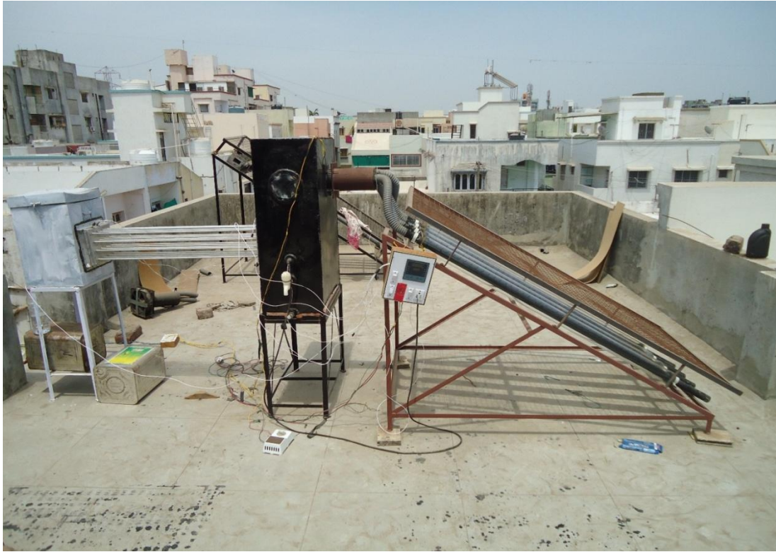
Figure3 Practical model of humidifier & dehumidifier for (CWOA) using circular solar collector of humidification-dehumidification process
