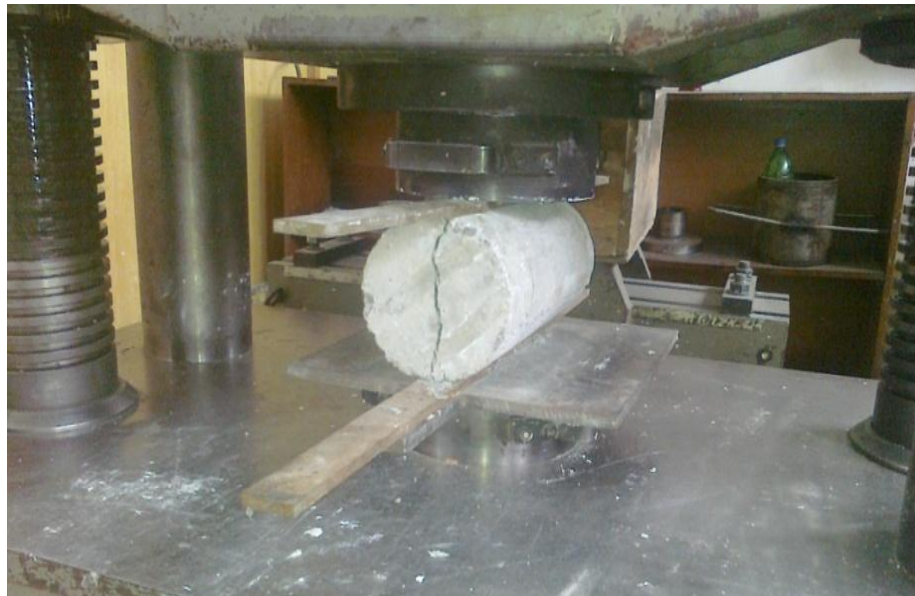
Figure 5: Split Cylinder Test for Hair Fiber Reinforced Concrete Cylinder in UTM
