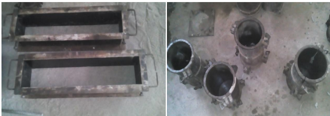
Figure 3: Reusable Molds of Beams and Cylinders Properly oiled.
