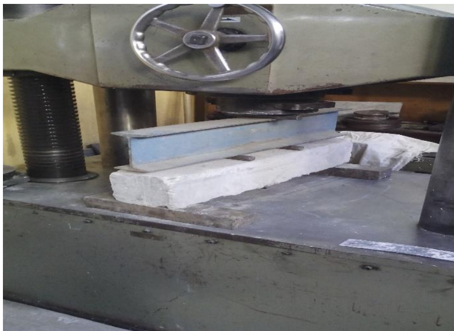
Figure 6: Flexural Test for Hair Fiber Reinforced Concrete beams in UTM
