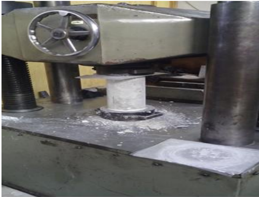
Figure 4: Compressive Strength Test for Hair Fiber Reinforced Concrete Cylinder in UTM
