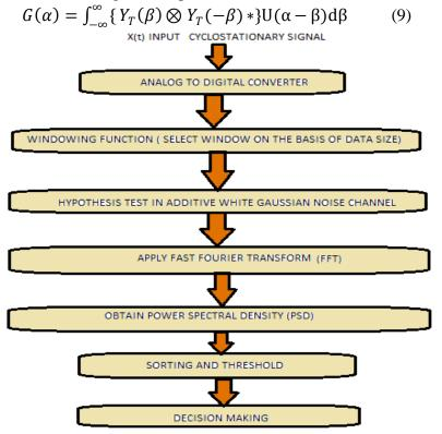
Figure 6. Flow chart of blind spectrum sensing for cyclostationary signal
