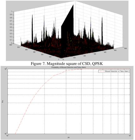
Figure 8. Probability of detection  $P_d$  and false alarm  $P_{fa}$ , QPSK, SNR=-20
