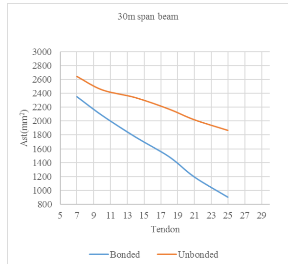
Figure 12. Extra reinforcement in 30m long span beam
