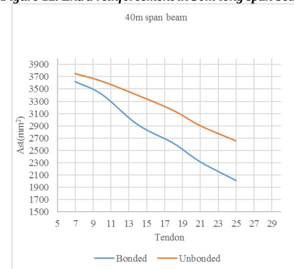
Figure 14. Extra reinforcement in 40m long span beam
