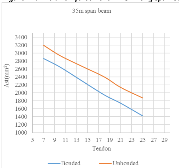
Figure 13. Extra reinforcement in 35m long span beam
