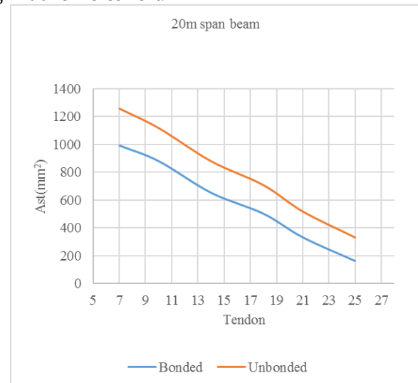
Figure 10. extra reinforcement in 20m long span beam
