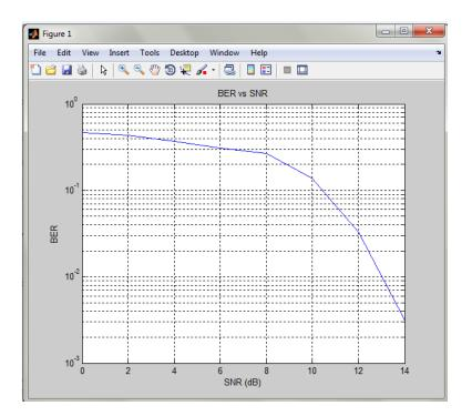
Figure.1 Bit Error Rate v/s Signal-to-Noise ratio.
