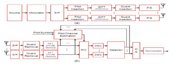
Fig. 1. Block diagram of the OFDM system, (a): Transmitter, (b): Receiver
