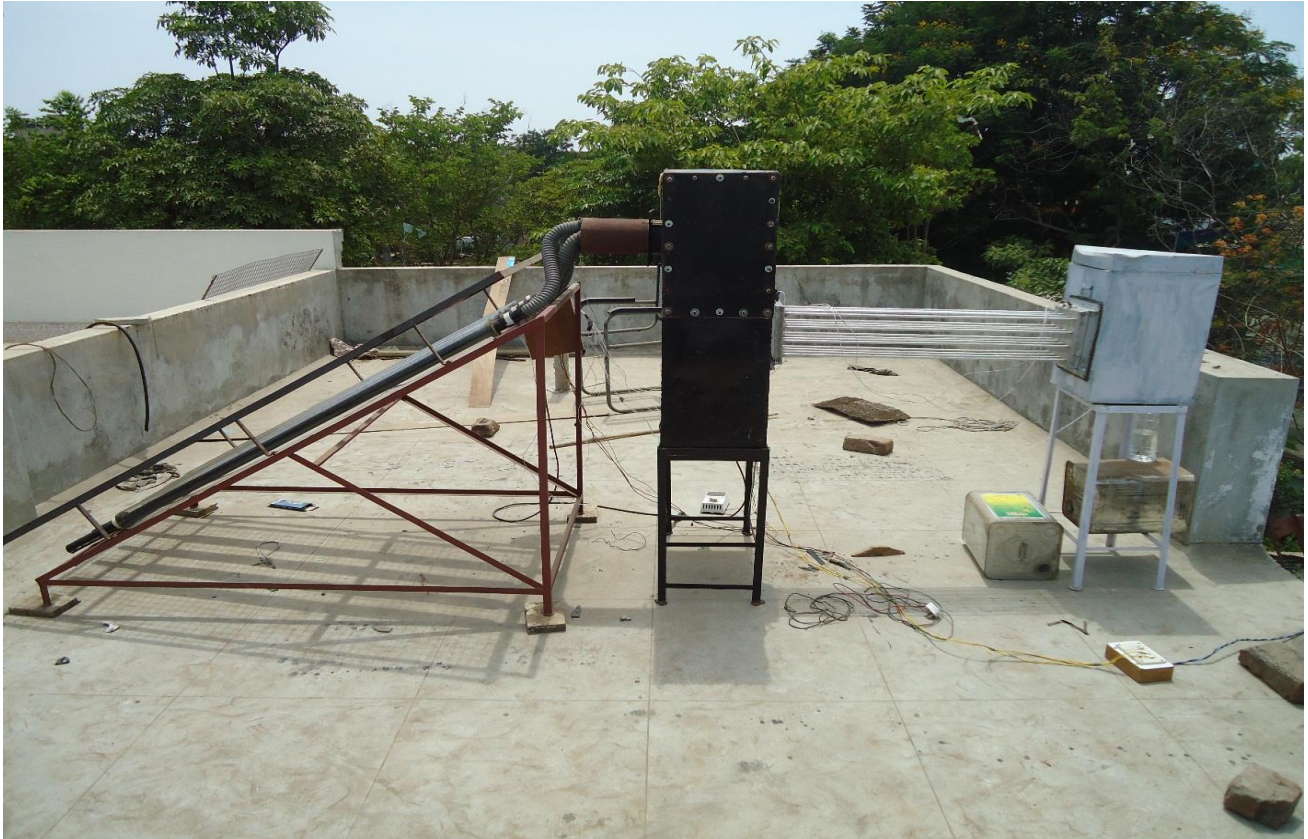
Figure 5 Experimental model of dehumidifier for (CWOA) using circular solar collector of humidification-dehumidification process
