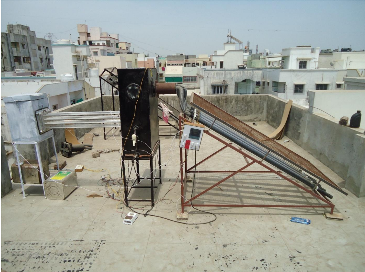
Fig 3 Experimental model of humidification chamber with the help of solar circular collector for close water open air system (CWOA) humidification dehumidification process
