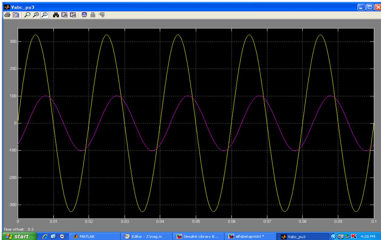
**Fig4.6 Voltage and Current waveforms for balanced linear load without compensation**
