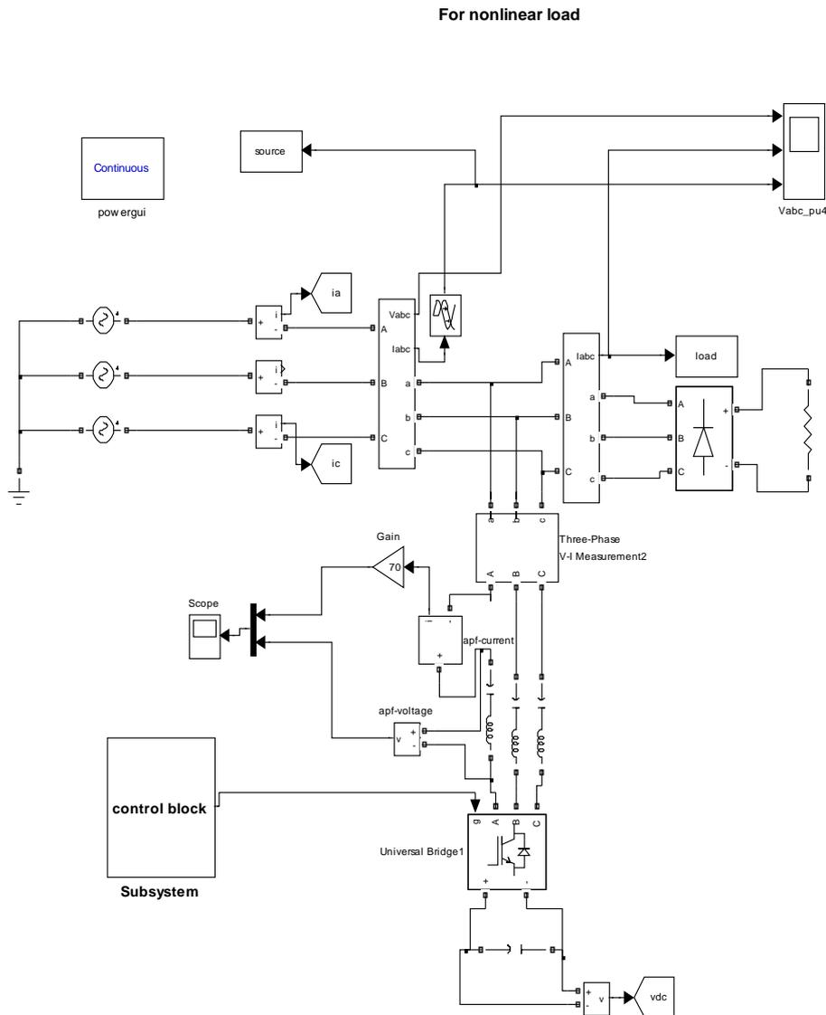
**Fig 4.1 simulink diagram for SVPWM based shunt Active Filter for non linear load**
