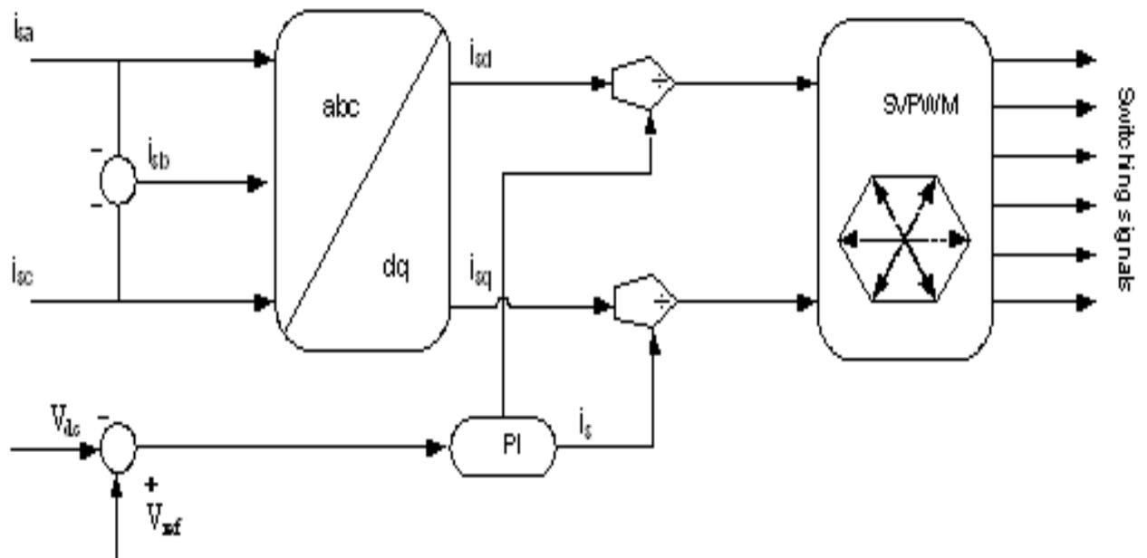
**Fig 4. Control Block Diagram of Proposed System**
