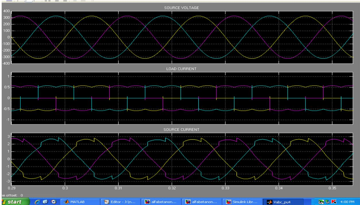
Fig 4.3 Wave-forms of source voltage, load current and source current for Non-linear load
