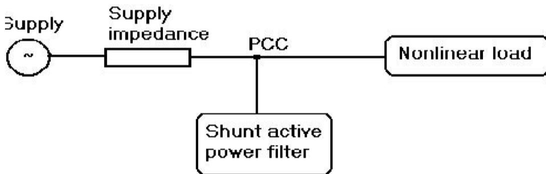
Fig. 1. Basic principle of shunt active power filter
