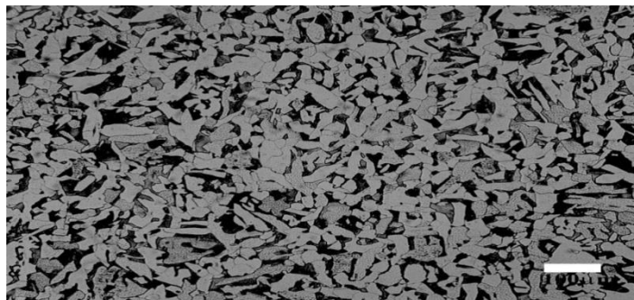
Fig. 9. Microstructure showing oriented cavities ferrite & pearlite in Convection superheater header
