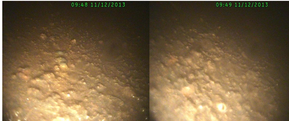
Fig. 10. Observation during Videoscopy foreign particles present in bed evaporator
