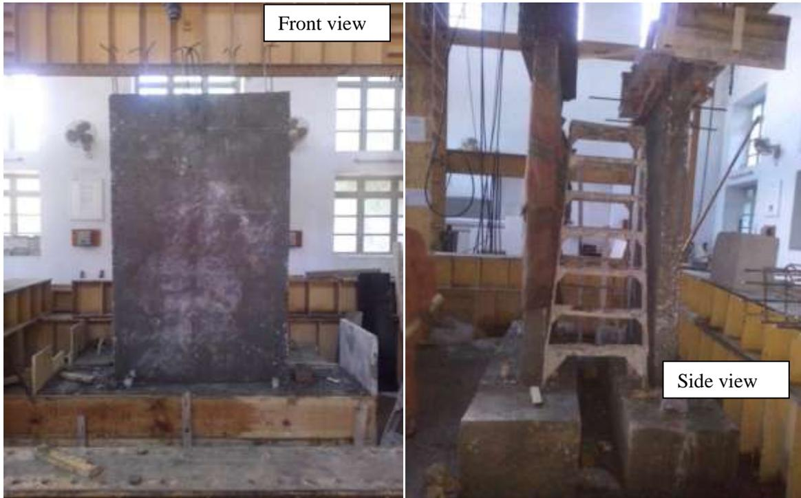
Figure 1: Construction of RC shear wall 1 & 2 in progress
