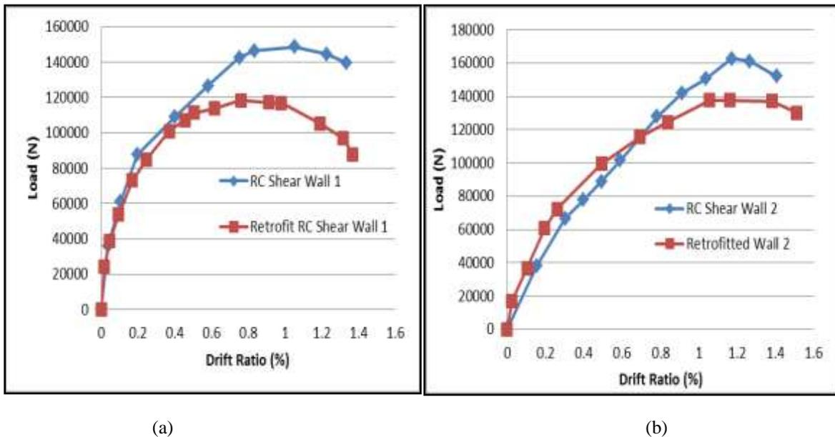
Figure 10: Load Comparison of Control and Retrofitted RC shear wall-1& 2
