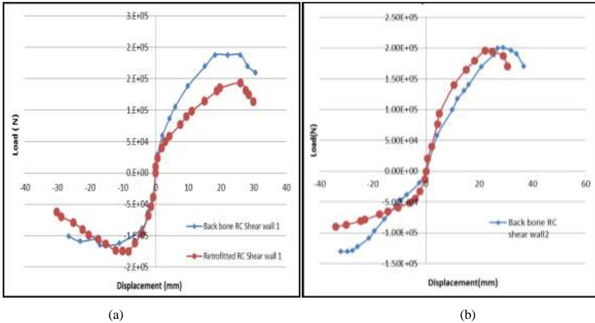
Figure 09: Comparison of Back bone curve of Original and Retrofitted RC shear wall-1& 2
