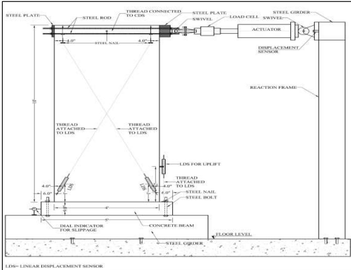
Figure 7: Detailed Experimental Setup for cyclic shear load test
