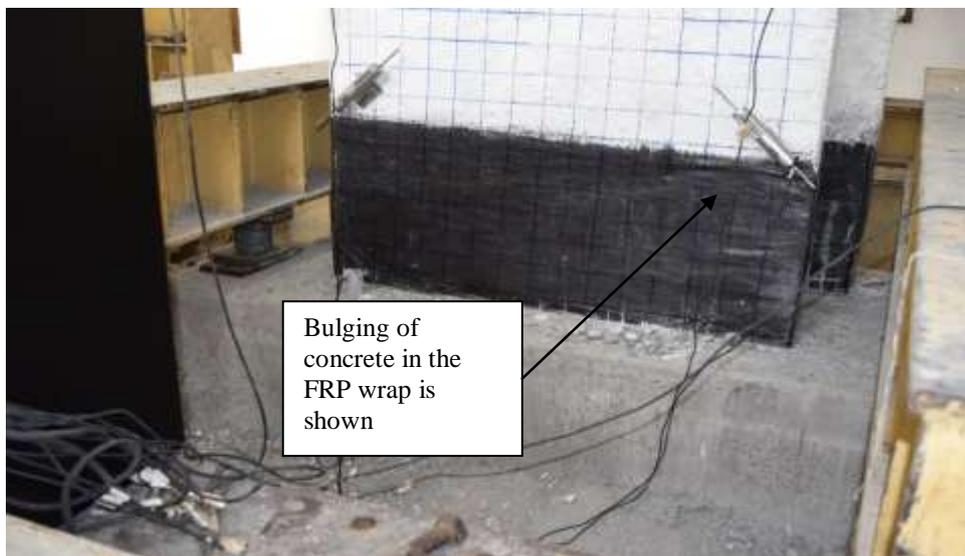
Figure 8: Bulging of Concrete in CFRP Wrap
