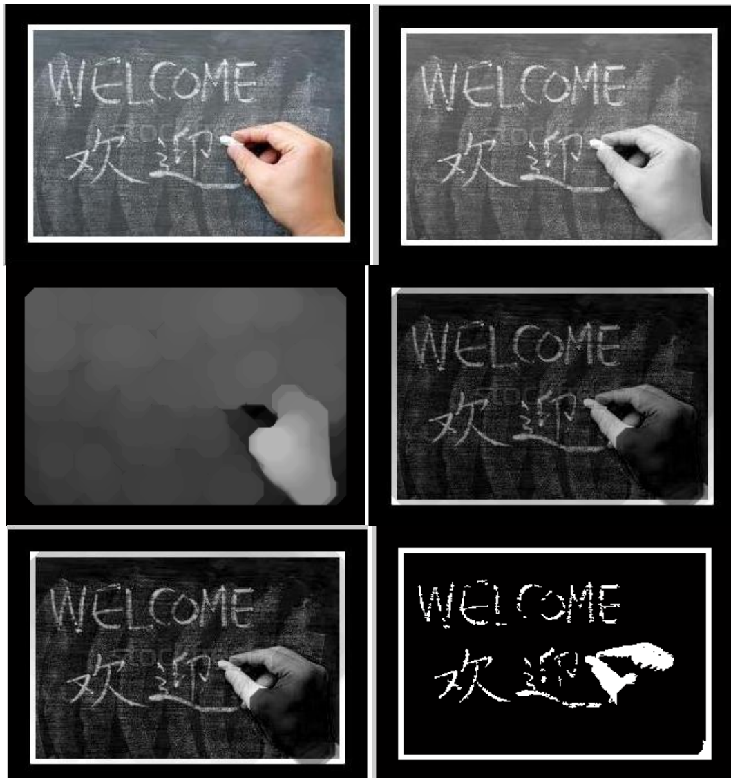
Figure8 left top – original test image, right top – gray scale image, middle right - original minus opened image, middle left - opened image, bottom left – contrast adjust image, bottom right – background cleared image
