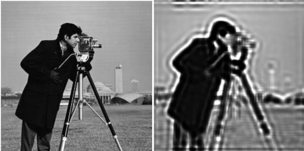
Figure3 left – original image, right– blind deconvolution[8]
