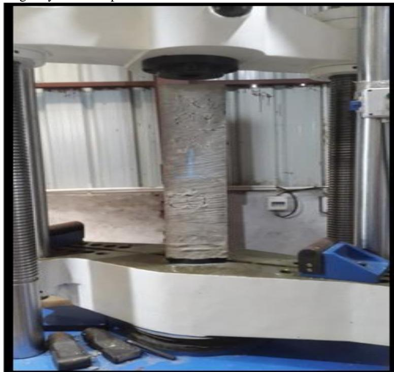
*Figure 1. Arrangement of column in UTM*
