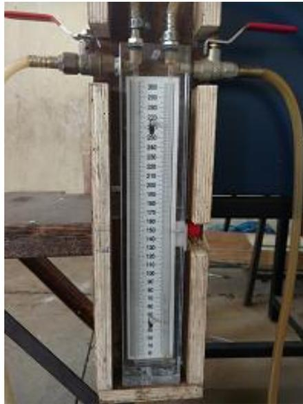
Fig (b) : Differential U- tube manometer
