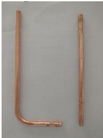
Fig.(a) : Simple pitot tube and Piezometric tube
