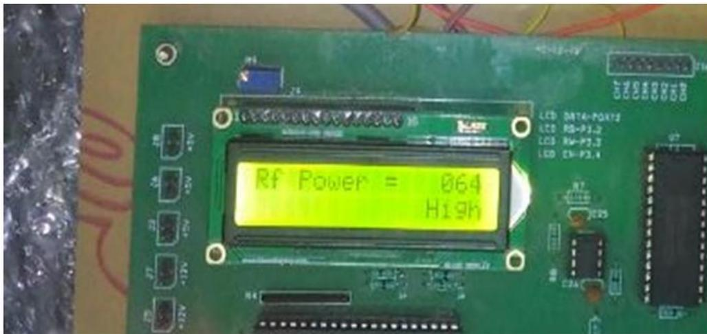
Fig.11.1 Due to incoming call RF signal is detected.
