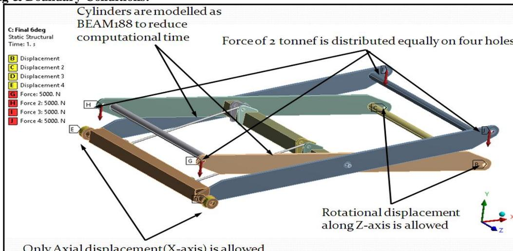
*Figure 4.3 Loading and boundary conditions*
