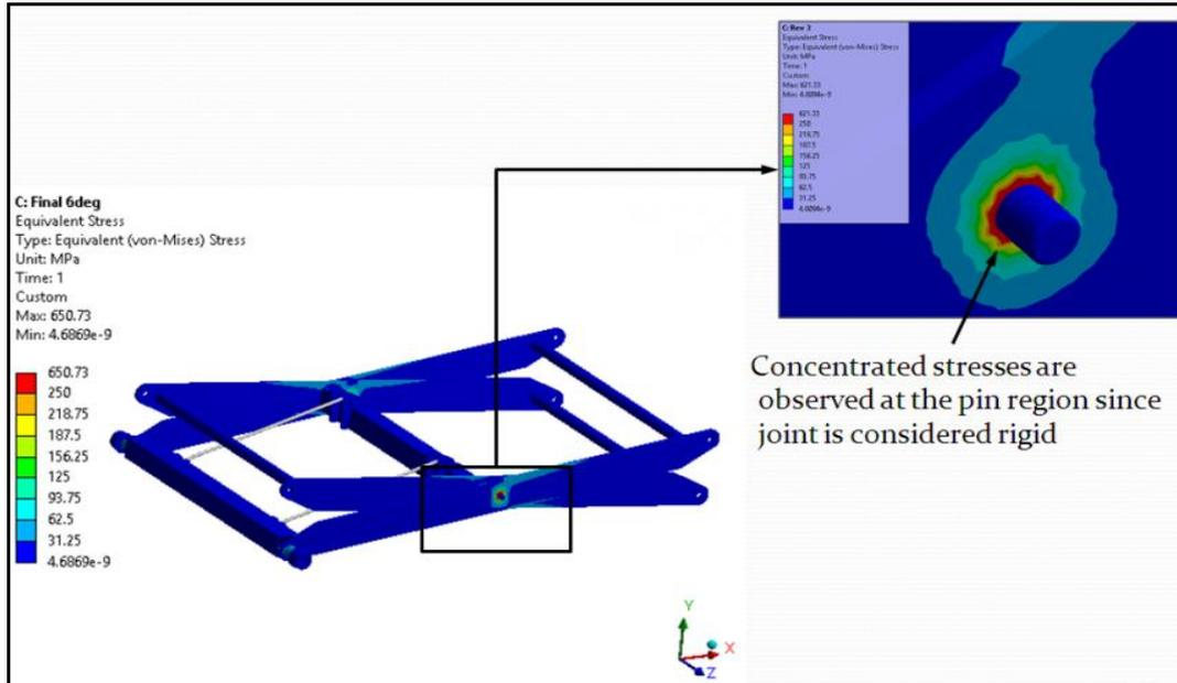
Figure 4.6 Equivalent stresses on lift
