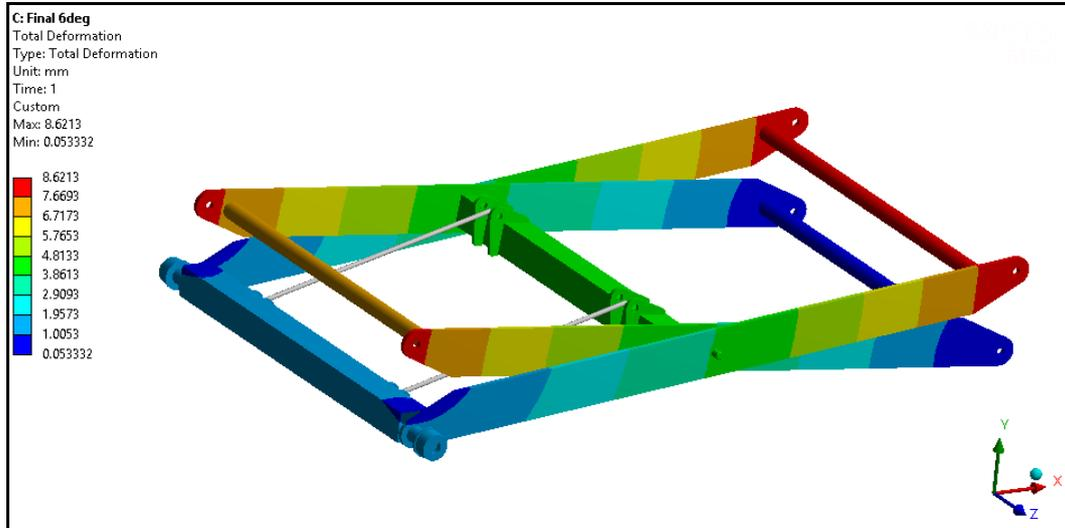
**Figure 4.4 Deformation of scissor lift**
