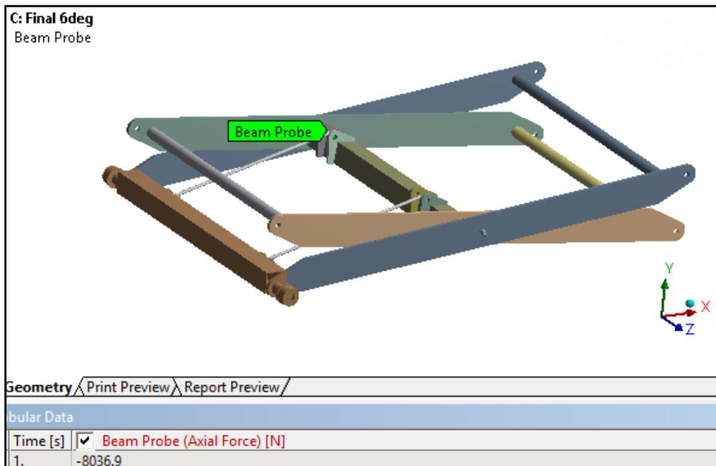
**Figure 4.5 Beam 188 reaction forces**
