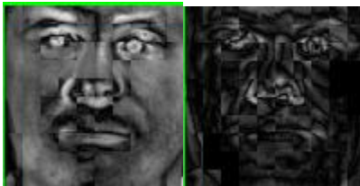
(c) Block eigen faces of data base images projected to eigen space(100 blocks - 10x10 sub image per block)
