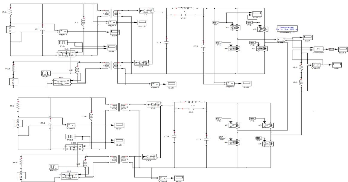
Figure 15. Simulink Model of Flyback with Cascaded Multilevel Inverter with RL Load
