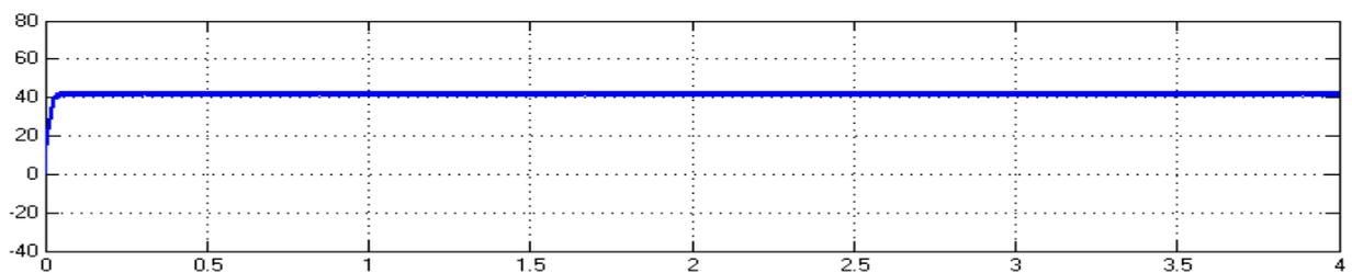
Figure 20. Output Voltage of Rectifier
