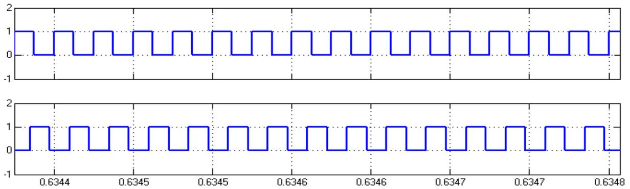
Figure 17. Switching Pulse for Flyback Inverter
