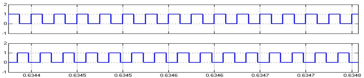
**Figure 6. Switching Pulse for Flyback Inverter**
