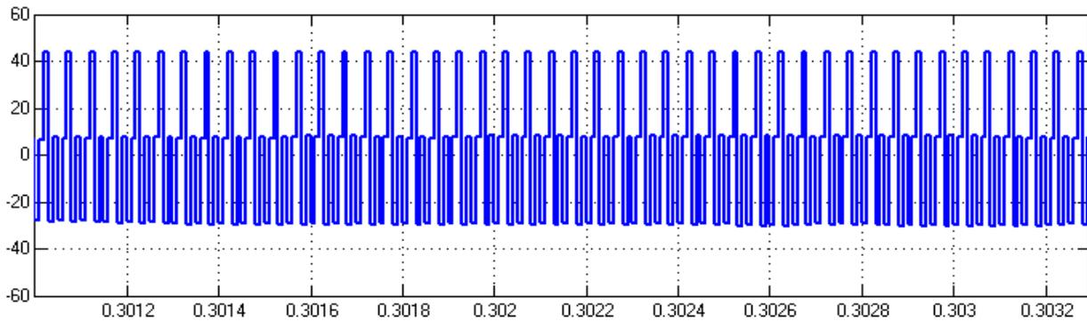
Figure 8. Transformer Secondary Voltage
