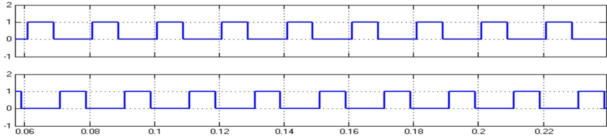
Figure 21. Switching Pulse for Multilevel Inverter (M1, M5)
