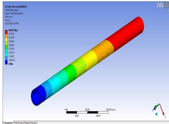
**Fig.5 Deformation diagram of composite drive shaft**
