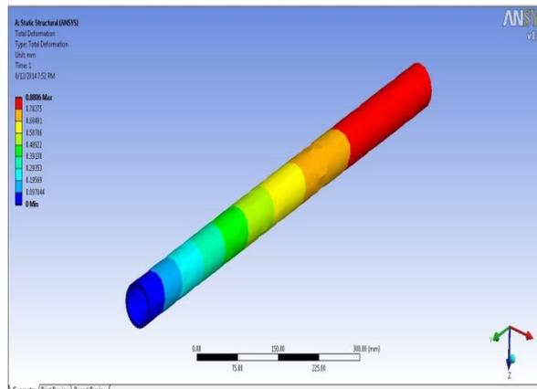
**Fig.4 Deformation diagram of steel drive shaft**
