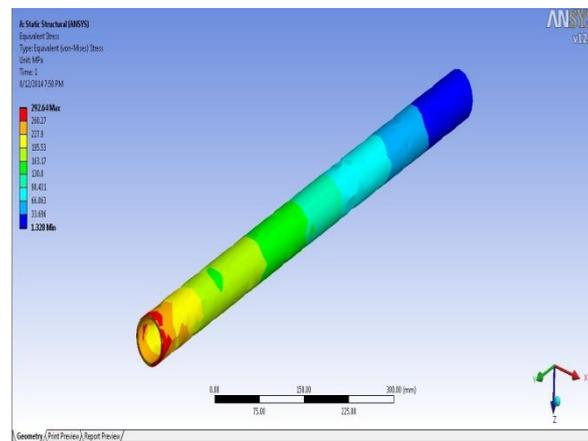
**Fig.6 Von misses stress diagram of steel drive shaft**
