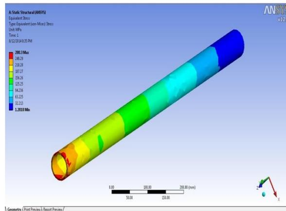
**Fig.7 Von misses stress diagram of composite drive shaft**
