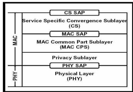
**Fig. 3: WiMAX Physical and MAC layer architecture**
