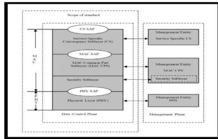
**Fig. 2: WiMAX Protocol Stack**
