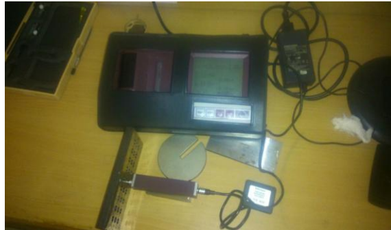
Fig 4 Mitutoyo Surface roughness test Model No SJ 304.design experiments are performed on the basis of level of cutting speed, feed rate and hole depth.
