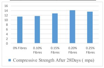
Figure: 5.4: compressive strength on 28 day Curing
