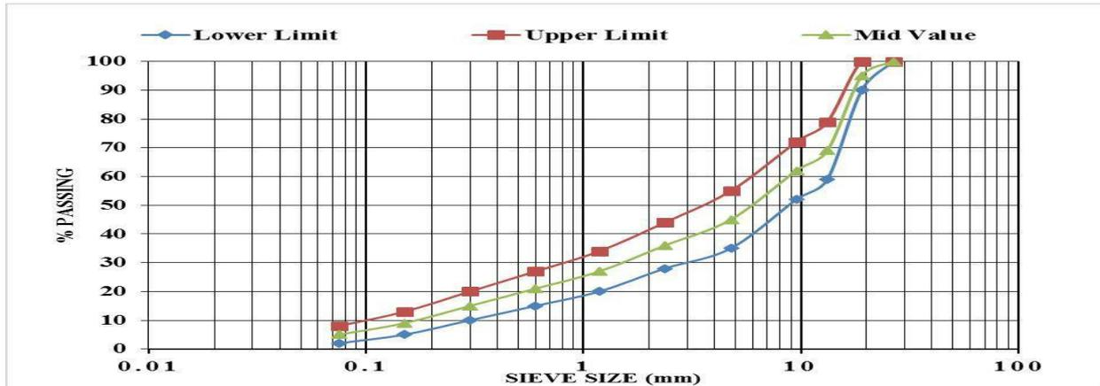
“Fig. 1 Aggregate Gradation of Bituminous Concrete (BC)-I Mix”
