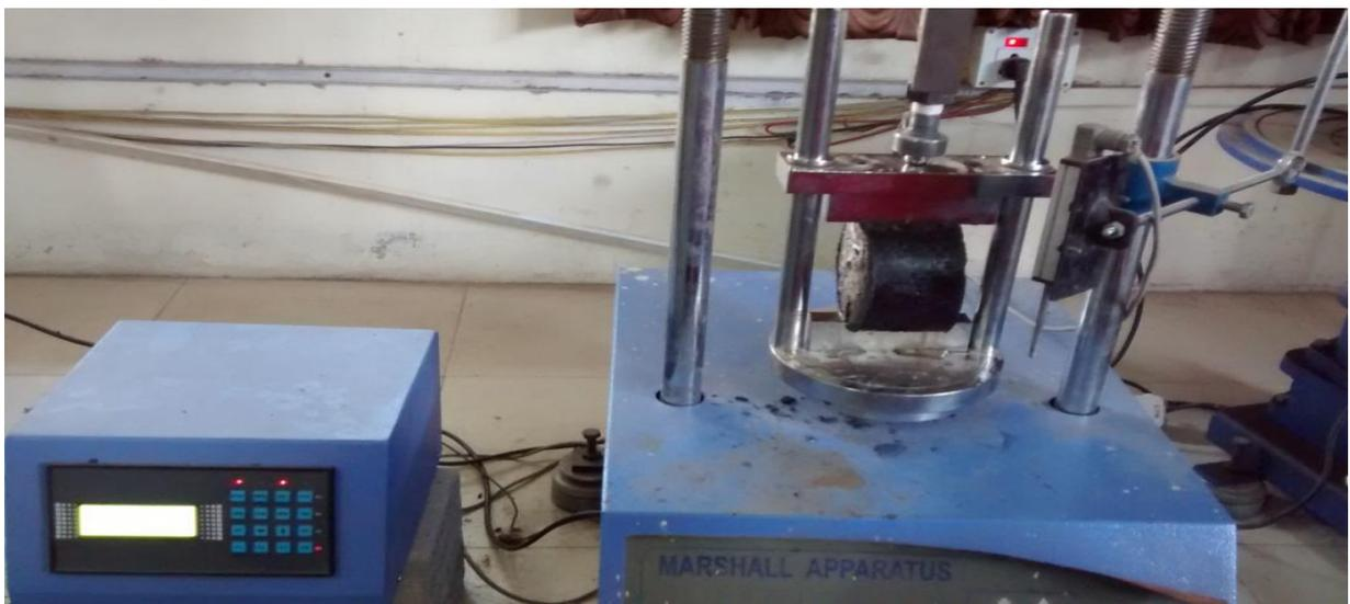
*“Figure 2 A View of Test setup of Indirect Tensile Strength”*
