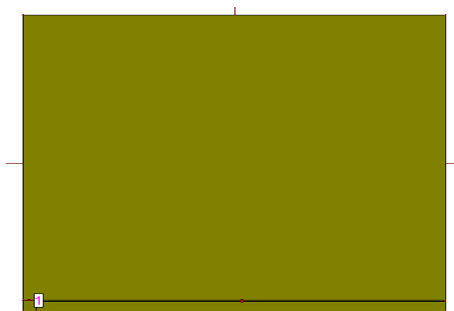
Figure 1. Proposed antenna geometry with Coaxial Feed at x,y(-17.5,-17.5)
