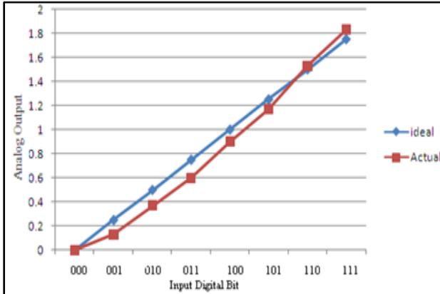
Figure 6: INL of Thermometer code DAC
