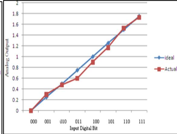
Figure 9: DNL of Thermometer code DAC
