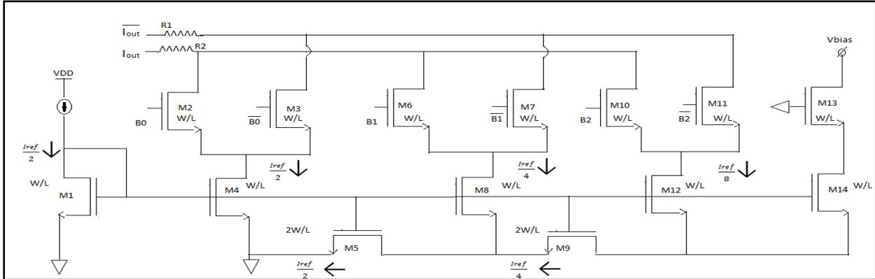
Figure 2: Binary-weighted current mirror, using w-2w topology
