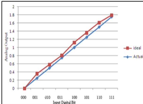
Figure 8: DNL of Current steering DAC
