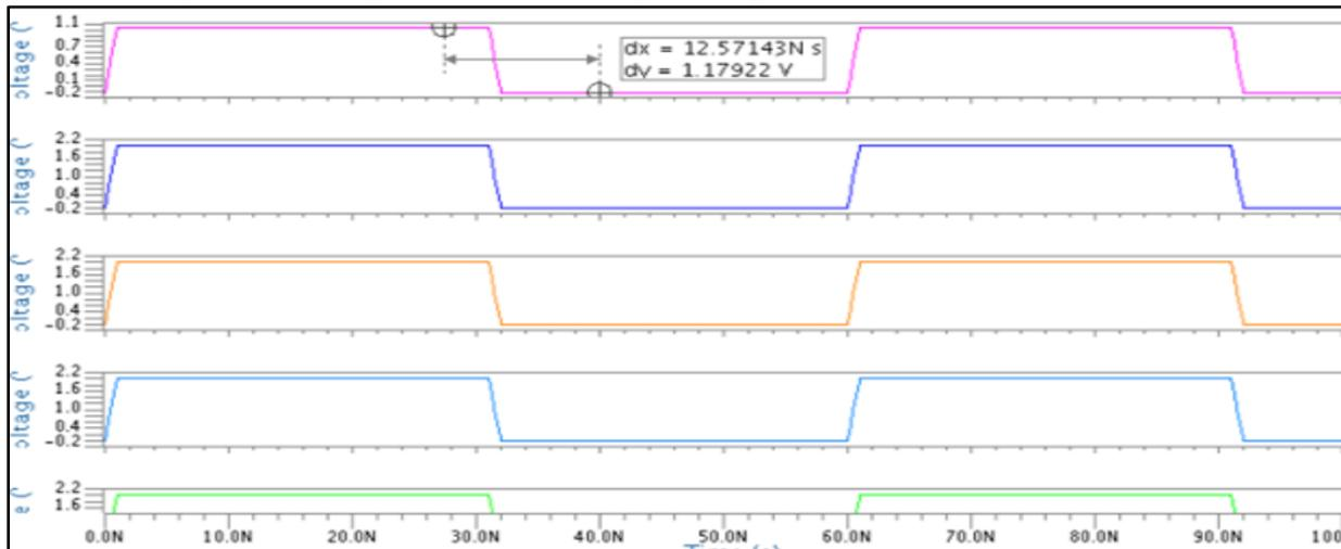
Figure 5: : input 0011111 and output is 1.17V for 3 bit Thermometer Code DAC
