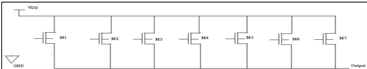
Figure 3: Thermometer Code DAC
