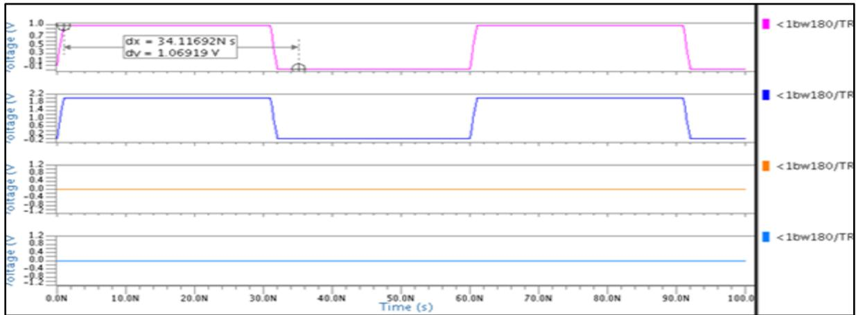
Figure 4: input 100 and output is 1.06V for 3 bit binary weighted Current steering w-2w
