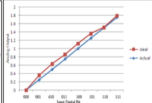
Figure 7: INL of Current steering DAC
