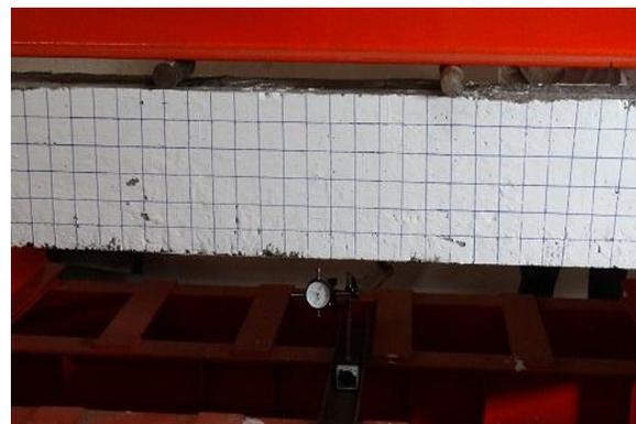
**“Figure 4. Arrangement of Dial Gauge at Mid-span”**
