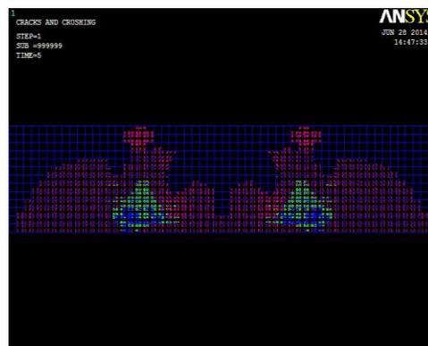
“Figure 19. Experimental and Analytical Crack pattern in Bottom Double Strip U Shaped Vertical Double Strip Beam - M25”
