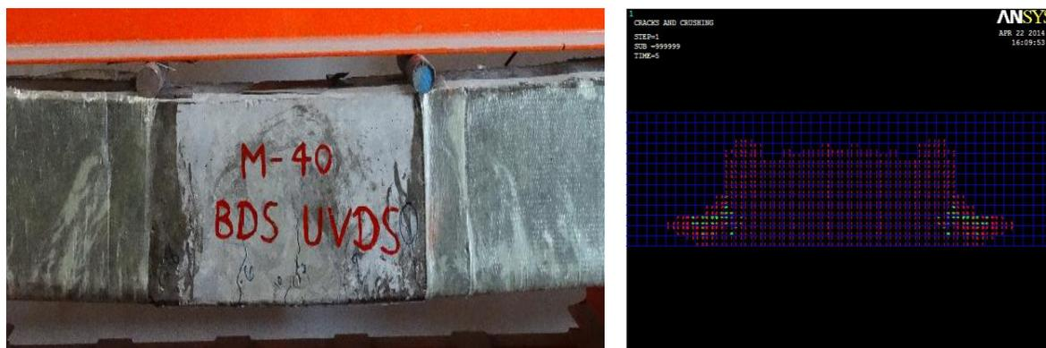
“Figure 22. Experimental and Analytical Crack pattern in Bottom Double Strip U Shaped Vertical Double Strip Beam – M40”
